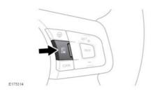
To switch between Speed limiter and Cruise control, press the **LIM** button on the steering wheel. These systems cannot be used simultaneously.
