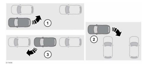
Park assist is an aid to maneuvering the vehicle in and out of parking spaces and parking bays. Park assist takes control of the vehicle's steering system to maneuver the vehicle.
