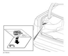
Turn the retaining lug, 90 degrees counter-clockwise, to release and then pull to lower.
