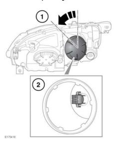
Rotate the appropriate headlamp cover, approximately 45 degrees counter-clockwise, to release and remove.
