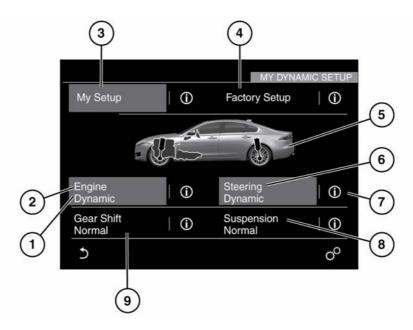
Vehicles with configurable dynamics, will allow the Dynamic driving mode settings to be configured via the Touch screen for selected characteristics, with a choice between Normal and Dynamic settings. See 120, TOUCH SCREEN CONTROLS to select this extra feature.
