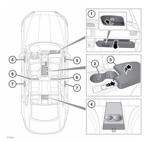
Glovebox: Pull the release handle to open. The glovebox can be locked/unlocked using the emergency key blade, mounted in the vehicle's Smart key. See 7, UNLOCKING THE VEHICLE.
