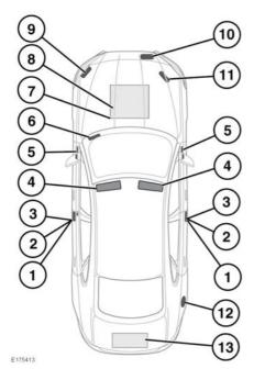
The vehicle weights and the Vehicle Identification Number (VIN) label: Located at the base of the driver's side B pillar. The VIN can also be shown in the Message center via the Vehicle Information and VIN Display menus. See 47, INSTRUMENT PANEL MENU.
