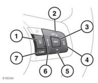
1. LIM: Press to switch between the speed limiters and ACC. The systems cannot be used simultaneously. The ACC warning lamp will illuminate when ACC is active. See 55, CRUISE CONTROL (GREEN).
