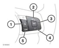
The Cruise control system is operated by controls mounted on the steering wheel. The driver can also intervene at any time, by use of the brake or accelerator pedals.
