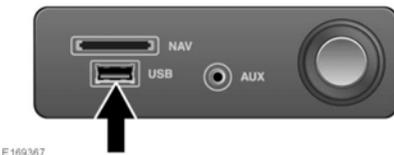
To initiate InControl Apps, connect your smartphone's USB cable to the vehicle's USB socket, located in the centre console cubby box. See **148, CONNECTING A MEDIA DEVICE**.
