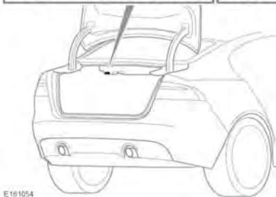
To install a SIM card, open the luggage compartment lid for access, then press the button (1) to release and remove the SIM card holder (2).
