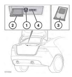
To install a SIM card, open the luggage compartment lid for access, then press the button (1) to release and remove the SIM card holder (2).
