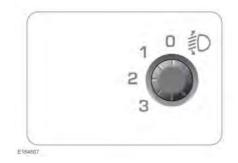
Use the rotary control to set the Halogen headlamps position to the correct level for the current vehicle load. This is located on the driver's side lower fascia.
