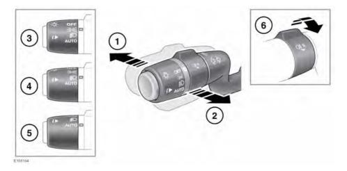
With the headlamps on, push the control away from the steering wheel to select high beam. The Instrument panel warning lamp will illuminate. See 54, HIGH BEAM (BLUE).
