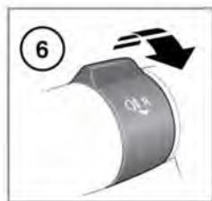
1. With the headlamps on, push the control away from the steering wheel to select high beam. The Instrument panel warning lamp will illuminate. See **54, HIGH BEAM (BLUE)**.
