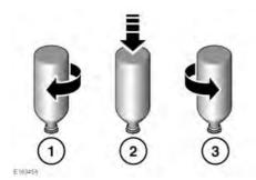
1. Place the refill bottle over the reservoir filler cap aperture and turn clockwise, until it is locked into position.
