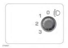
Use the rotary control to set the Halogen headlamps position to the correct level for the current vehicle load. This is located on the driver's side lower fascia.
