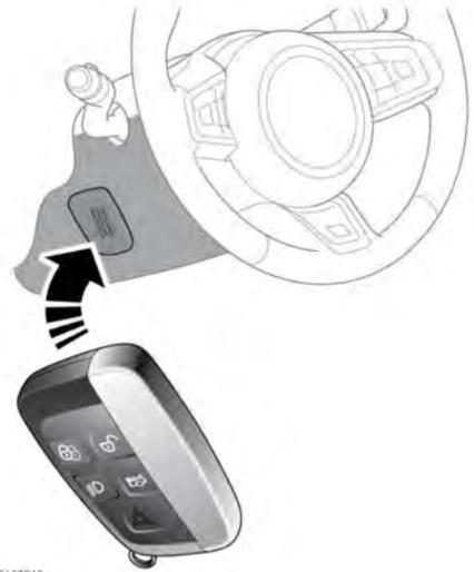
1. Position the Smart key flat against the side of the steering column, with the buttons facing outwards.
