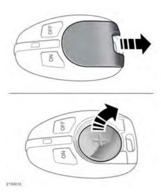
With the front of the remote control facing upwards, press down on the rear of the access cover and push completely off to reveal the battery compartment. Note that the battery should be inserted with the positive side facing upwards. Remove the old battery and making sure that the correct polarity is maintained, insert a new, unused 3 volt CR2032 battery. Align and push the cover back to the original position.
