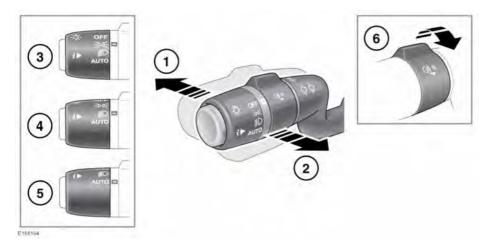
With the headlamps on, push the control away from the steering wheel to select high beam. The Instrument panel warning lamp will illuminate. See 55, HIGH BEAM (BLUE).
