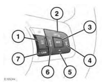
1. LIM: Press to switch between Speed limiter and ACC. The systems cannot be used simultaneously. The ACC warning lamp will illuminate when ACC is active. See 54, CRUISE CONTROL (GREEN).
