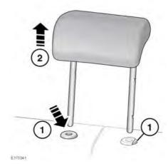
To remove the head restraint, raise the head restraint to its uppermost position.
