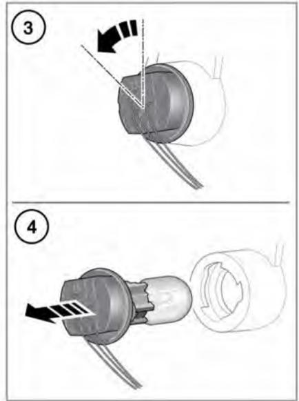
Reverse the removal procedure to install a new bulb.
