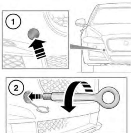
The front towing point is located behind a small access panel in the front bumper.
