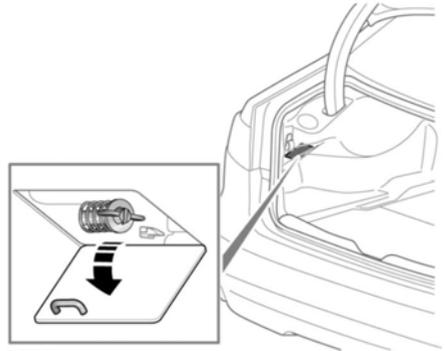
Turn the retaining lug, 90 degrees counter-clockwise, to release and then pull to lower.
