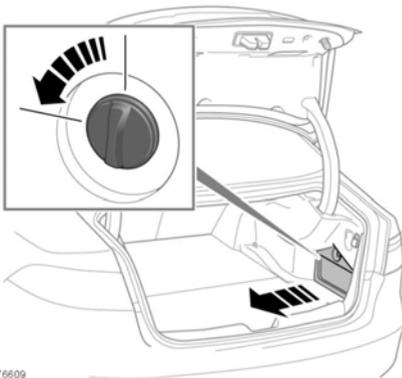
Turn the retaining lug, 90 degrees counter-clockwise, to release, then lower and lift to remove.
