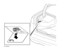
Turn the retaining lug, 90 degrees counterclockwise, to release and then pull to lower. Reverse the removal procedure to refit.
