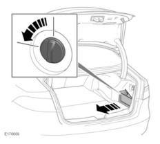
Turn the retaining lug, 90 degrees counterclockwise, to release, then lower and lift to remove.
