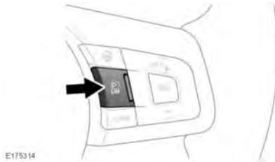
To switch between the Speed limiter systems and the Cruise control systems, press the **LIM** button on the steering wheel. These systems cannot be used simultaneously.
