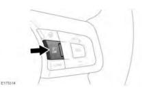
To switch between the Speed limiter systems and the Cruise control systems, press the **LIM** button on the steering wheel. These systems cannot be used simultaneously.
