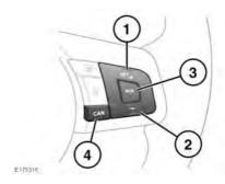
1. **SET+**: Press to set or increase the speed limit. The set-speed limit will be displayed in the Message centre.
