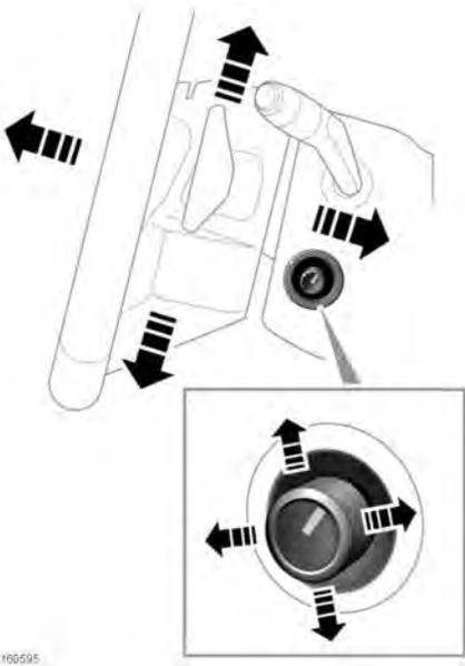
Vehicles with an electric steering column, can be adjusted to alter the tilt and reach of the steering wheel:
