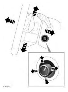
Vehicles with an electric steering column, can be adjusted to alter the tilt and reach of the steering wheel:
