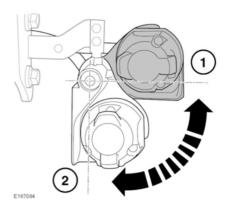
The detachable tow ball's trailer socket should be manually deployed (2) and stowed (1), as illustrated.
