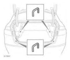
Securing points are provided in the luggage area to assist in safely securing items.
