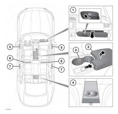
Glovebox: Pull the release handle to open. The glovebox can be locked/unlocked using the emergency key blade, mounted in the vehicle's Smart key. See 6, UNLOCKING THE VEHICLE.
