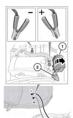
Open the bonnet and locate the engine compartment front fuse box. See **229**, **FUSE BOX LOCATIONS**.
