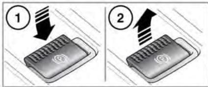
1. With the ignition switched on, press the brake pedal and press down on the EPB switch. This will release the EPB.
