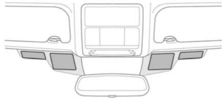
Electronic actuating cards, such as toll road payment cards or Radio Frequency (RF) ID tags, can be fixed at the dedicated locations on the inside of the windscreen. If these cards are located at any other part of a solar attenuating windscreen, the electronic scanners may not recognise them.
