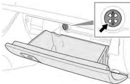
The glove box temperature can be controlled using the vent located in the glove box. Rotate counter-clockwise to open, or clockwise to close the vent.
