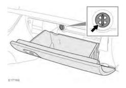
The glove box temperature can be controlled using the vent located in the glove box. Rotate counter-clockwise to open, or clockwise to close the vent.
