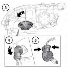
*Note:* Note the orientation of the bulb holder to aid refitting.
