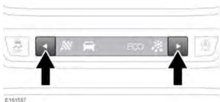
Use the buttons, located on the centre console (see **302, DRIVER CONTROLS**), to move through the different driving modes. The currently selected driving mode's LED indicator lamp will illuminate to confirm the selection. The Message centre will also display the relevant driving mode icon (except for Normal mode) and a temporary confirmation message.
