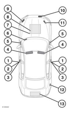
1. The vehicle weights and the Vehicle Identification Number (VIN) label: Located at the base of the driver's side B pillar. The vehicle build-date plate (Australian vehicles only) will also be located here.
