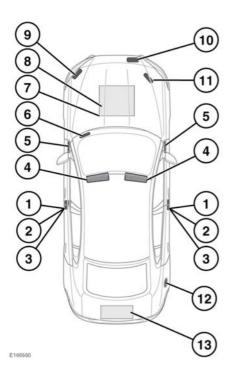
The vehicle weights and the Vehicle Identification Number (VIN) label: Located at the base of the driver's side B pillar. The vehicle build-date plate (Australian vehicles only) will also be located here.
