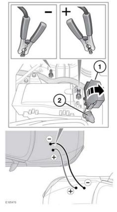
Open the bonnet and locate the engine compartment front fuse box. See 214, FUSE **BOX LOCATIONS.** Release the 2 covers to access the positive boost point terminal:
