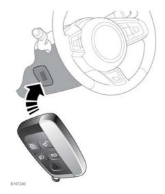
1. Position the Smart key flat against the side of the steering column with the buttons facing outwards.
