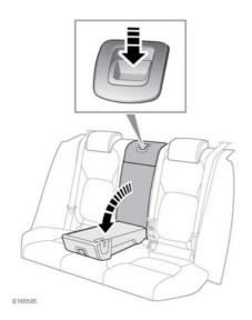
The middle seatback can also be released separately. Press and hold the button to release and then fold the middle seatback forward.
