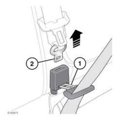
The rear centre seat belt can be released from its buckle, before folding the rear seatback/s, to allow for improved access to the Luggage compartment.
