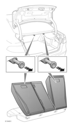
**Note:** The folding rear seats are not available on all vehicles. It is dependent on the vehicle specification.
