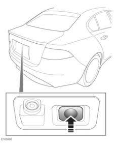
To open the luggage compartment, press the luggage compartment exterior release button (arrowed), if the vehicle is not locked. Alternatively, press the relevant Smart key button. See **6**, **UNLOCKING THE VEHICLE**.
