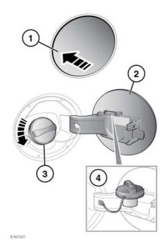
The vehicle must be unlocked using the Smart key, before the filler flap can be opened.
