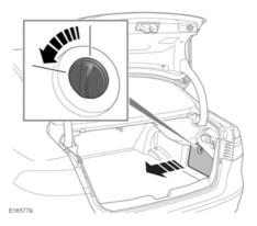
Turn the retaining lug, 90 degrees counter-clockwise, to release, then lower and lift to remove.
