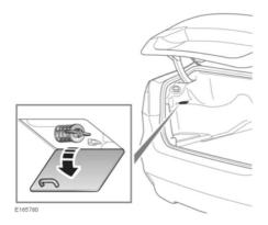
Turn the retaining lug, 90 degrees counter-clockwise, to release and then pull to lower.
