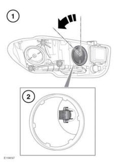
Rotate the headlamp cover, approximately 45 degrees counter-clockwise to release and remove.
