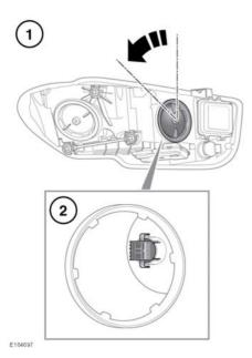
Rotate the headlamp cover, approximately 45 degrees counter-clockwise to release and remove.
