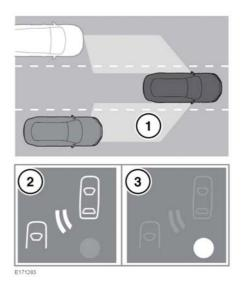
The Blind Spot Monitor (BSM) system monitors a zone that covers the area adjacent to the vehicle, that is not easily visible to the driver. The system uses a radar on each side of the vehicle to identify any overtaking vehicle/object within the blind spot area (1) of the vehicle, while disregarding other objects which may be stationary or travelling in the opposite direction, etc.
