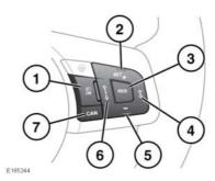
LIM: Press to switch between the Automatic Speed Limiter (ASL) and ACC. The systems cannot be used simultaneously. The ACC warning lamp will illuminate when ACC is active. See 54, CRUISE CONTROL (GREEN).
