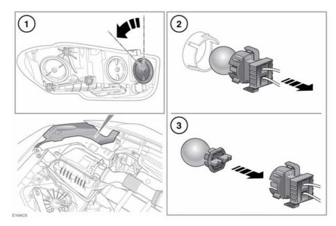
Rotate the headlamp cover, approximately 45 degrees counter-clockwise to release and remove.
