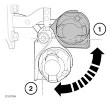
The detachable tow ball, trailer socket should be manually deployed (2) and stowed (1), as illustrated.
