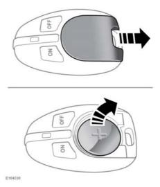
With the front of the remote control facing upwards, press down on the rear of the access cover and push completely off to reveal the battery compartment. Note that the battery should be inserted with the positive side facing upwards. Remove the old battery and making sure that the correct polarity is maintained, insert a new, unused 3 volt CR2032 battery. Align and push the cover back to the original position.
