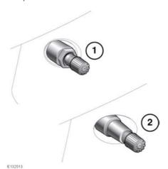
Wheels fitted with a TPMS can be visually identified by the external metal lock nut and valve (1). All Jaguar non-TPMS wheels have a rubber valve fitted (2).
