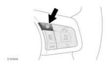
To activate the heated steering wheel, press the switch. Press again to switch off.
