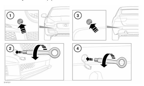
The towing eye is part of the vehicle's tool kit, located under the luggage compartment floor panel. For vehicles supplied with a spare wheel, see 236, WHEEL CHANGING. For vehicles supplied with tyre repair kit, see 231, TYRE REPAIR KIT.
