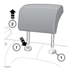
To remove the head restraint, raise the head restraint to its uppermost position.
