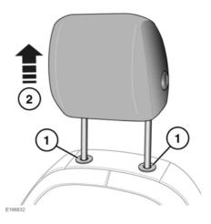
To remove the head restraint, raise the head restraint to its uppermost position.
